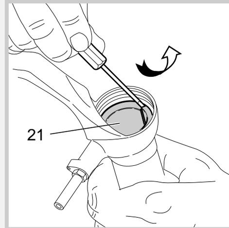
**PUMPING ROD DISASSEMBLY**
